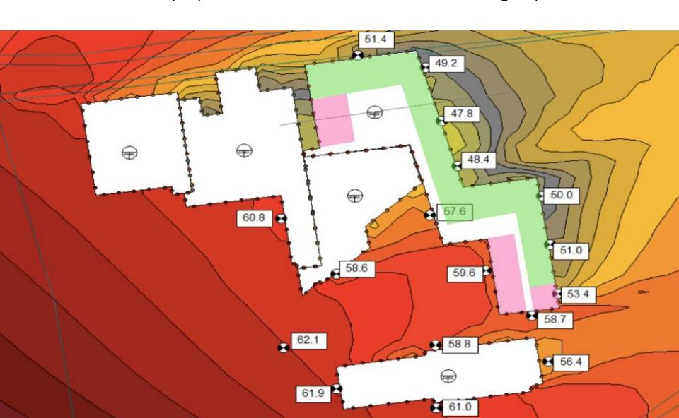
Mechanical ventilation system removed through detailed noise mapping
