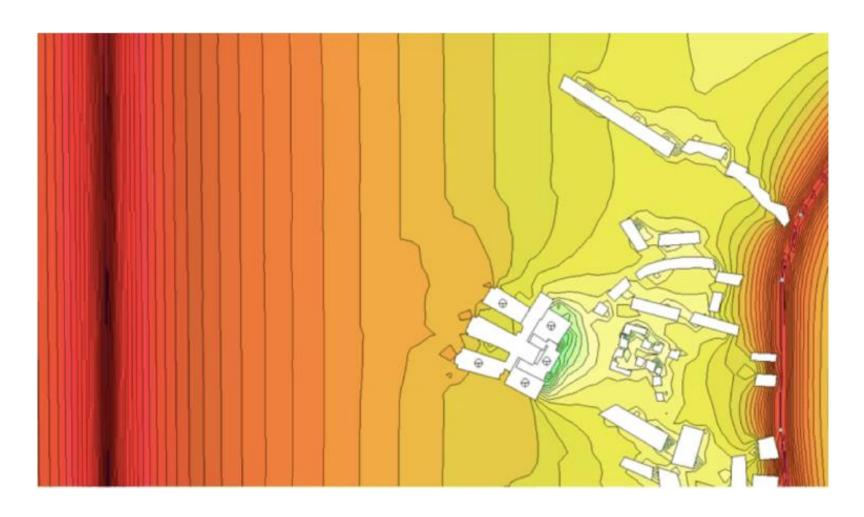
Establishing the sound angle of a noise source through noise mapping
