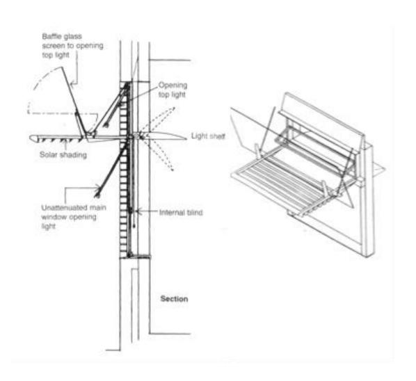
Normal openable window 10-15 dB of sound reduction
