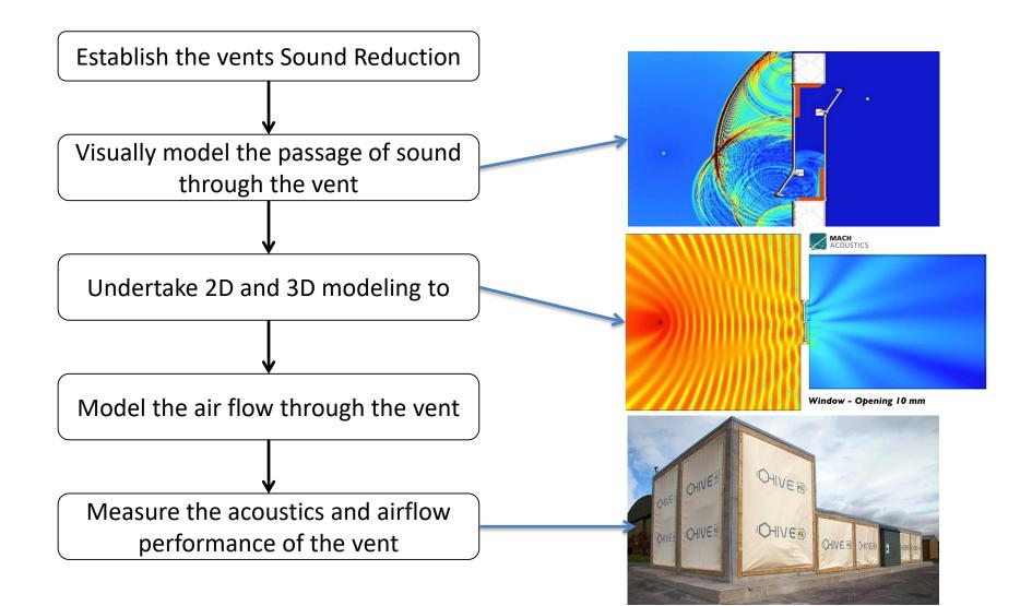
Acoustic vent & loudspeaker shaping
