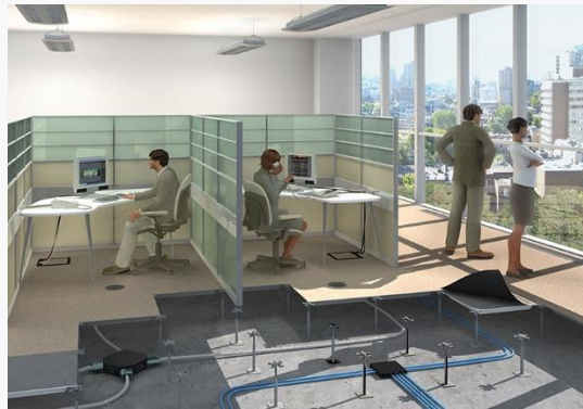
Under Floor Air Distribution (UFAD) System
