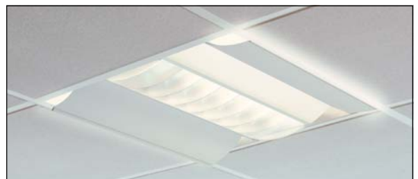
Recessed luminaire for DSE environments with increased upward light component using 40 or 55 W compact fluorescent lamp; LOR: 77.6% Luminaire lumens per circuit watt (55 W lamp and class A2 ballast): 59.8
