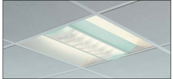
Recessed luminaire for DSE environments with decorative feature using 40 or 55 W compact fluorescent lamps; LOR: 80% Luminaire lumens per circuit watt (40 W lamp and class A2 ballast): 62.2
