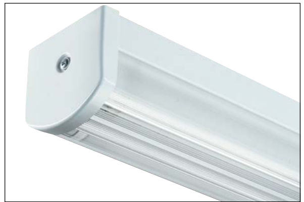
Luminaire with prismatic controller for one or two linear 28 or 35 W T5 high efficiency lamps; LOR 95% for single lamp version and 86% for twin lamp version Luminaire lumens per circuit watt (single 28 W lamp, class A2 ballast): 77.2 Luminaire lumens per circuit watt (twin 28 W lamps, class A3 ballast): 65.8
