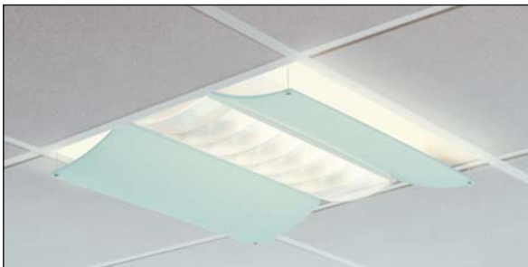
Recessed luminaire for DSE environments with glass feature giving a small upward light component using 40 or 55 W compact fluorescent lamp; LOR: 75.8% Luminaire lumens per circuit watt (40 W lamp and class A2 ballast): 59
