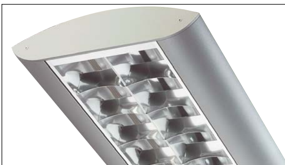
Individually suspended direct/indirect luminaire for two 28 or 35 W T5 lamps high efficiency lamps, maximum surface luminance below 1500 cd/m 2 ; LOR: 91% Luminaire lumens per circuit watt (35 W lamp, class A2 ballast): 77 Luminaire lumens per circuit watt (28 W lamp, class A3 ballast): 69.6
