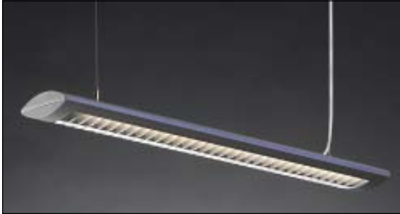
Slim pendant luminaire with parabolic louvre for 2 x 28W T5 lamps and CDELMA class 2 ballast, LOR: 86% Luminaire lumens per circuit watt: 72
