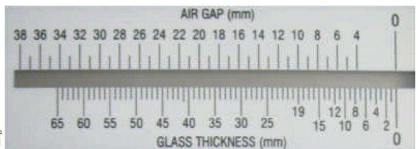
nesses and air gap width with access from inside the building only. Record whether the glazing can be replaced from inside or outside.
