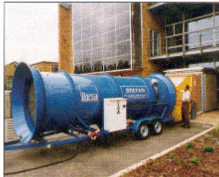
**The BRE pressure testing its new Environmental Building. This rig will also be used to pressure test the PROBE 2 buildings.**
