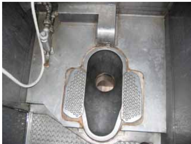
The latest in In-train toilet facilities – don't look too carefully but you can see the train track through the outlet hole. Picture taken on a train travelling through the jungles of Malaysia.
