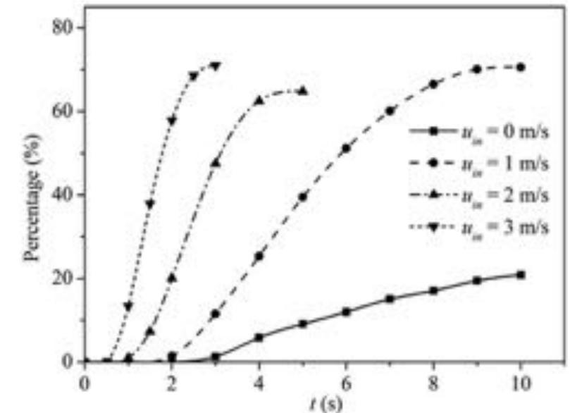
Effect of evaporation and air speed on droplet size
