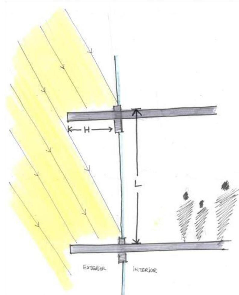
Initial Sketch Demonstrating Shading Principle
