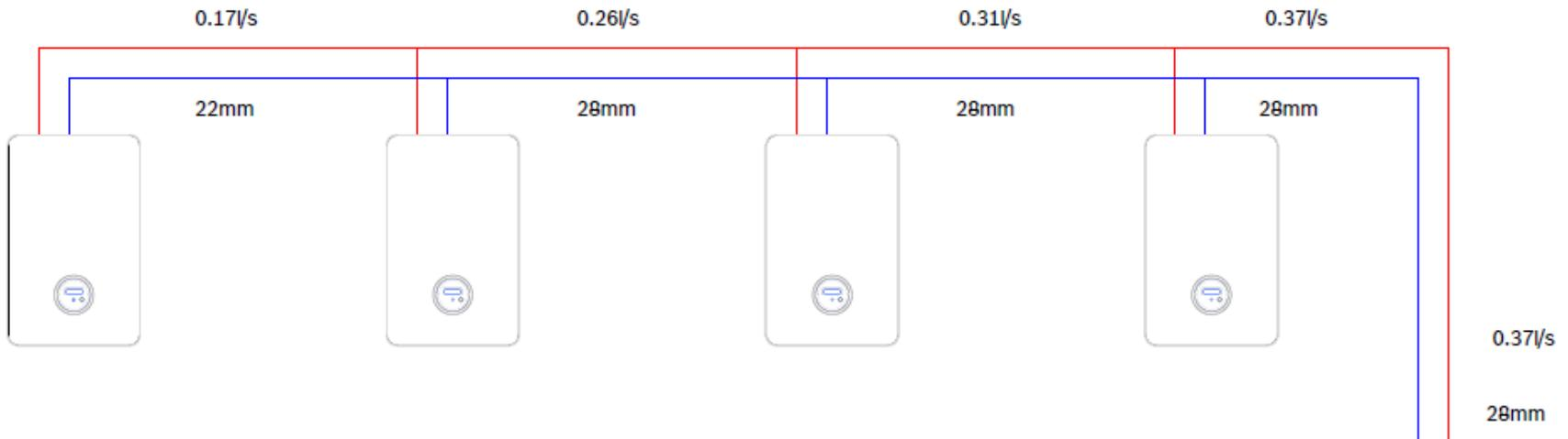
Pipe sizing start point 250Pa/m max, but iterative process required to look at least life cycle cost (CP1 3.6)
