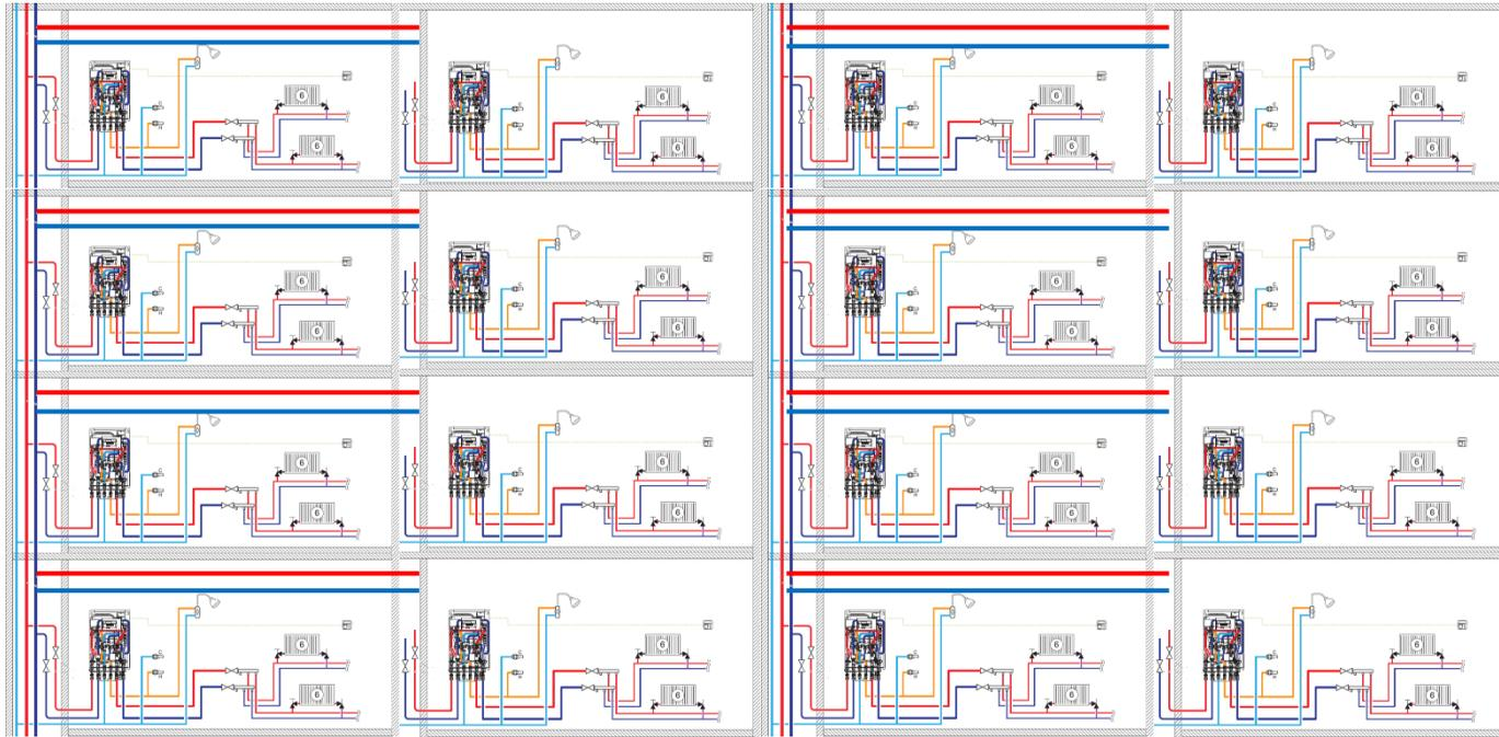
Minimise lateral runs as these lead to greater heat losses
