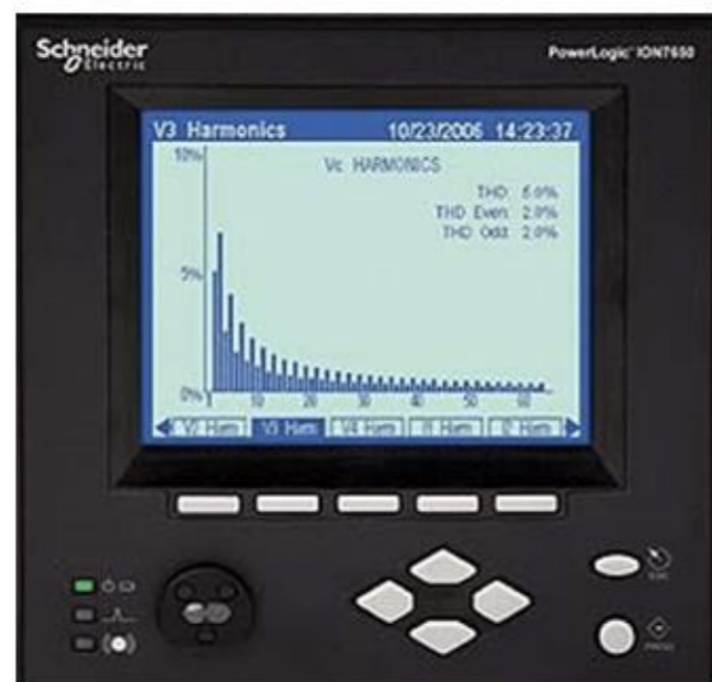
Fig.9 THD indicator measurement by power quality metering
