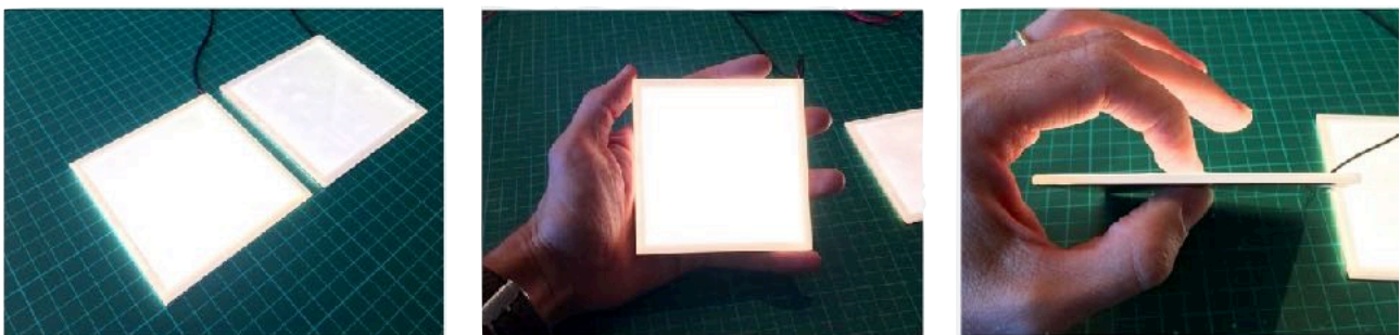
Figure 2: Ultra-Thin LED Light Modules by Lightly Technologies
