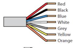
Power 24V GND Analog GND Control signal Feedback signal T1 or resistance input T2 or resistance input Available I/O:
