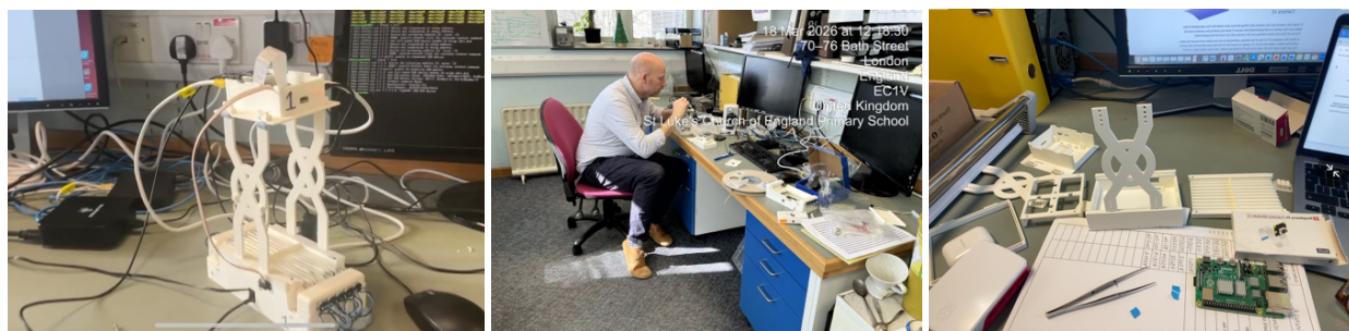
Figure 5. The building process of the Ethoscope behavioral monitors, designed to monitor the movement and sleep of the flies over several days.
