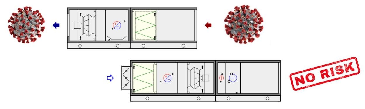
Exhaust Air Transfer Ratio (EATR) is 0% in this configuration
