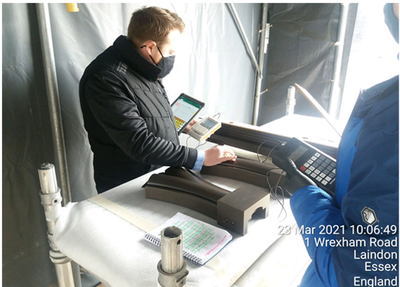
IMG10 – Third party inspection for the first batch of aluminium cladding components completed by The Paint Specialist
