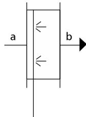
Page 3-121 Appendix 3.A2: humidification — sprayed coil process: paragraph 2 of remarks should read: 'Saturation efficiency is of the order of 80–90%. Water quality is of the order of 0.5–1.0 litre·s<sup>-1</sup> per m<sup>3</sup>·s<sup>-1</sup>. Air velocity of the order of 2.5 m·s<sup>-1</sup>.'
