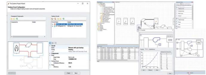
Figure 4.7 Illustration of 'template' and 'detailed' HVAC system modelling in TAS software (courtesy of EDSL)
