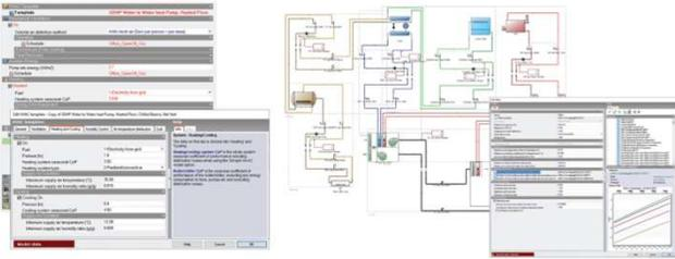
Figure 4.5 Illustration of 'template' and 'detailed' HVAC system modelling in DesignBuilder software (courtesy of DesignBuilder Software)
