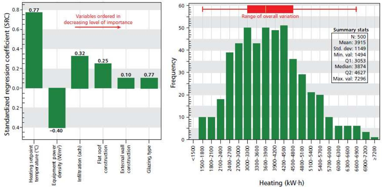
Figure 7.5 Example of parametric sensitivity and uncertainty analysis (courtesy of DesignBuilder Software)
