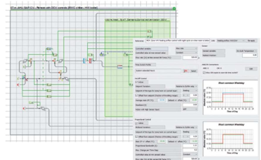
Figure 4.6 Illustration of 'template' and 'detailed' HVAC system modelling in IES software (courtesy of IES)
