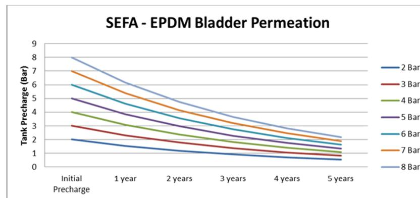
**Conclusion:** These figures are relevant as they show the air loss rates of the Italian and Turkey bladder tanks and present further evidence that bladder tanks are leaking air at high rates through permeation alone. When coupled with air loss at the flange, the total precharge air loss is much higher and thus requires the customer to check and maintain the air precharge at regular intervals.
