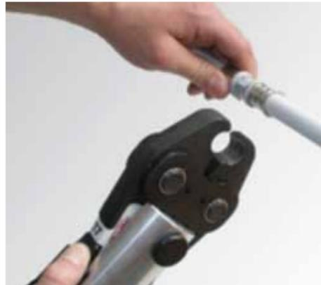
Press Fit jointing has been used on the continent for much longer and is more widely used than the UK. Initially in the UK it was thought of as expensive because of the investment in the press tooling required to do the fittings, but with no hot works allowed on many sites press fit is becoming the preferred alternative.
