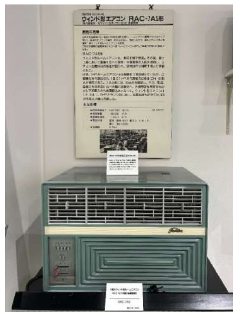
Figure 2 As Japan was recovering from the war, a room air conditioner development project was launched at Toshiba's Yanagimachi Factory. The RAC-7A5 was introduced to the market in 1958, the first domestically produced 1 horsepower window air conditioner. Photo by William Holley (02.04.25)
