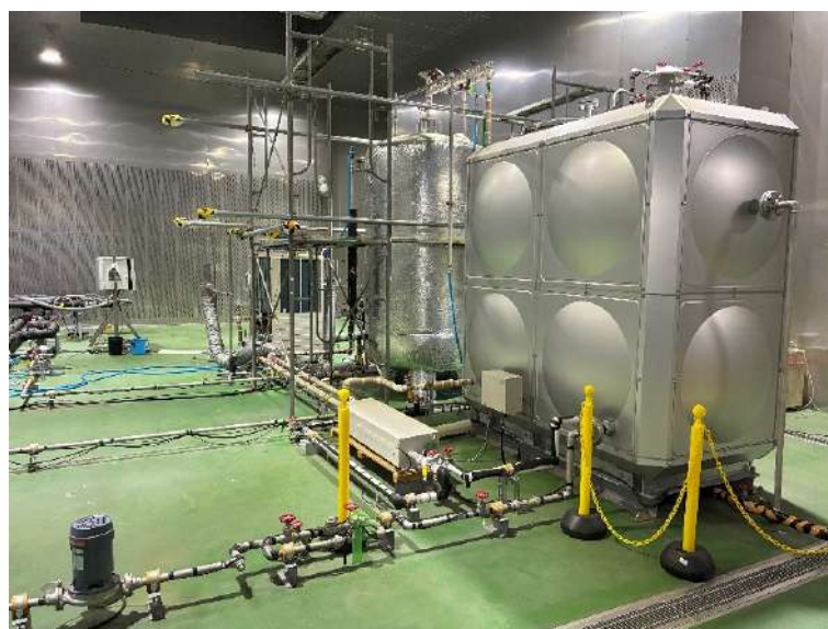
Figure 22: CRIEPI Testing Facility, external VRV unit test. This laboratory can simulate an external environment (-20 to 50°C).
