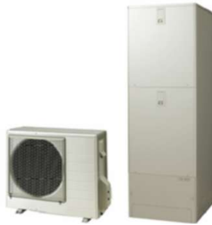
Figure 15 Eco Cute Heat Pump for Hot water generation. A typical HP capacity of 4.5kW is combined with a hot water tank of 300 litres
