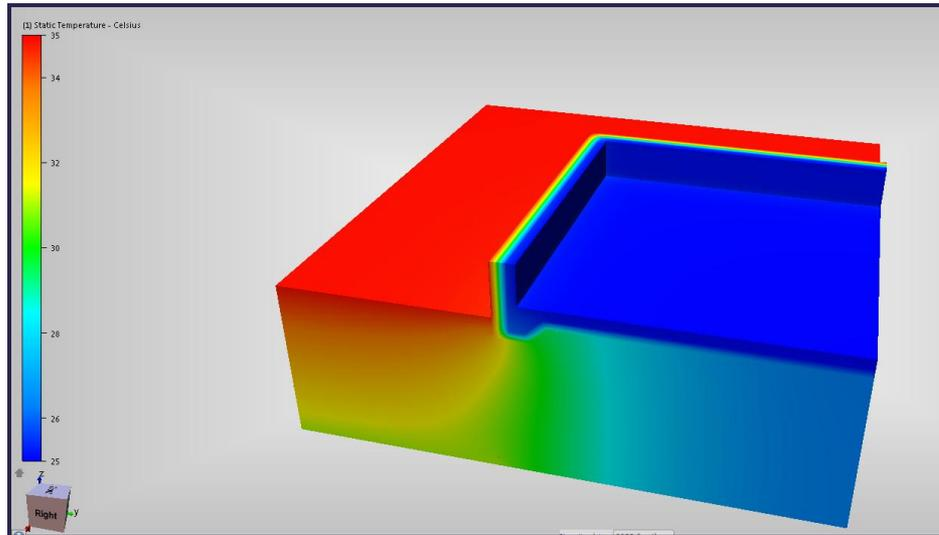
Images shows cut-away of conduction model of wall and ground floor for average summer conditions
