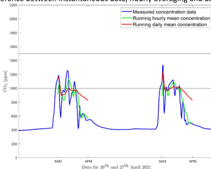
Figure 1: Carbon dioxide concentrations in a classroom with uncontrolled natural ventilation. The instantaneous CO<sub>2</sub> concentration are plotted in blue, during occupied hours<sup>17</sup> running hourly mean concentrations are plotted in green and the running daily average (i.e. since 09:00) are plotted in red.
