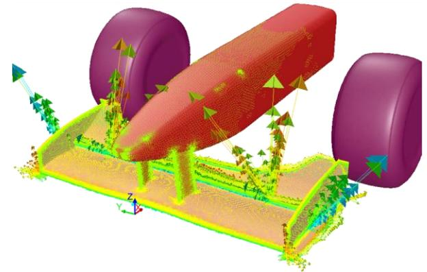
Once the adjoint solution is computed it can be used to guide intelligent design modifications to a system by a simple gradient algorithm for design optimization.
