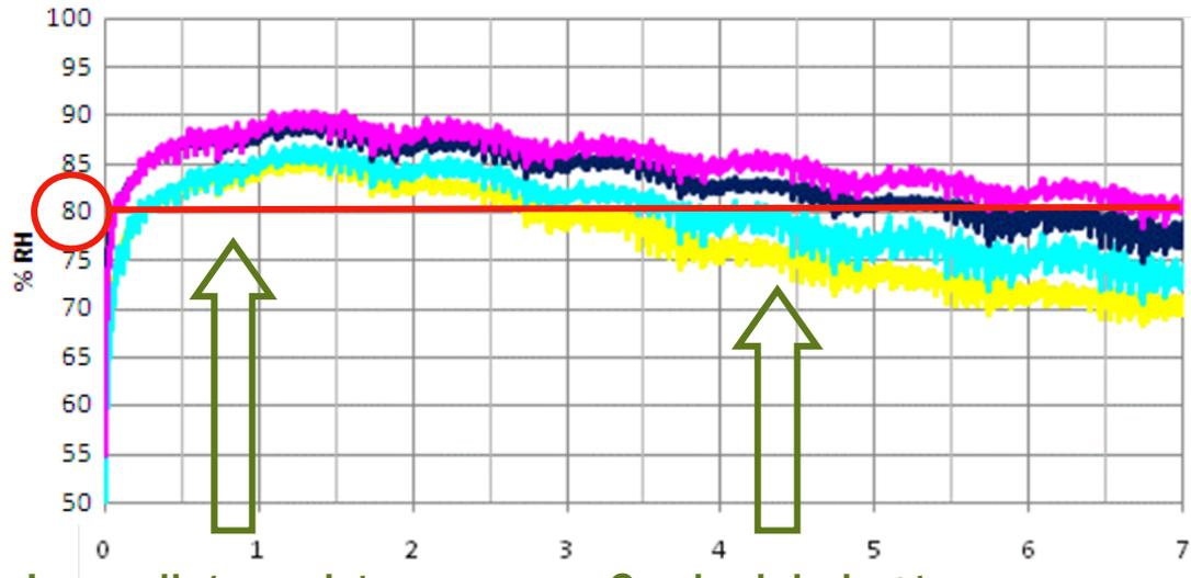
Immediate moisture accumulation on cold plaster due to internal insulation
