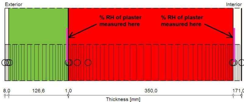
External wall insulation on solid brick
