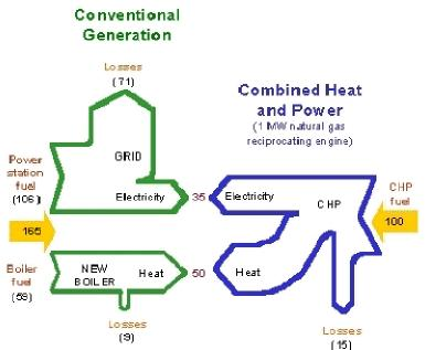
In its simplest form, CHP refers to combined heat and power (or cogeneration), which means using the waste heat from the prime mover to satisfy the heating and/or domestic hot water needs of buildings or processes. However, sometimes CHP has also been used to denote combined cooling, heating, and power (CCHP), or trigeneration, as depicted on the next graphic.
