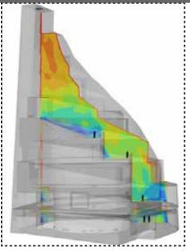
proposed design would deliver good airflow to all areas, therefore providing adequate thermal comfort for occupants during both peak summer and winter conditions. Fluent CFD software was used for the analysis due to its ability to deal with complex geometry and multi-physics
